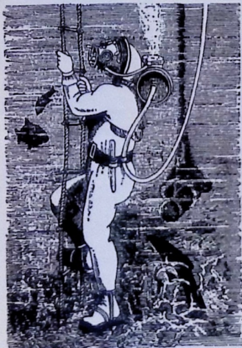
The Rouquayrol-Denayrouze apparatus was the first regulator to be mass produced (from 1865 to 1965)
